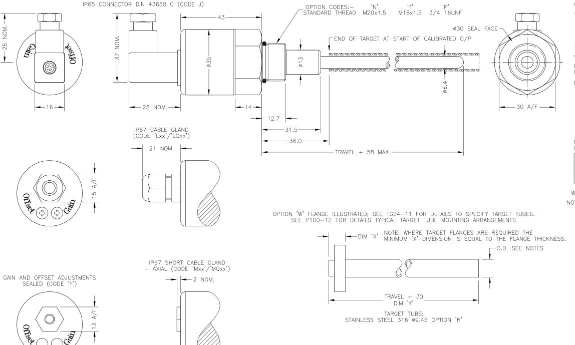
ELECTRICAL OPTIONS/ SPECIFICATIONS <u>OUTPUT</u> **SUPPLY** 0.5 TO 4.5V RATIOMETRIC 5V SUPPLY CURRENT 12mA TYP. 20mA MAX. CABLE:  $0.2 \, \text{mm}^2$ , 0/A SCREEN, PUR JACKET — SUPPLIED WITH 50cm OR REQUIRED LENGTH IN cm (15000cm MAX). STANDARD 3-CORE: JACKET Ø4mm BLACK e.g. 'L50' OPTIONAL 5-CORE: JACKET Ø4.6mm BLUE e.g. 'LQ50' CABLE/CONNECTOR\* CONNECTIONS; 3 CORE 5 CORE CONNECTOR RED RED ORG +SENSE (5-WIRE ONLY) BLACK BLACK OV GRY -SENSE (5-WIRE ONLY) WHITE WHITE OUTPUT SCREEN SCREEN BODY
